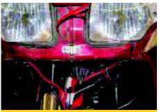
I fed a long cable tie around between the headlights to secure the wiring and inverters inside the fairing.
