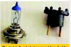
The stock bulb and adapter removed from the bike.
