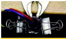
I used vice grip pliers to hold the alignment tabs together, then I laid the pliers on the bench with the bulb hanging off the edge.
