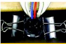
I filled around the base of the new bulb with sealant and allowed it to fully cure before disturbing it.
